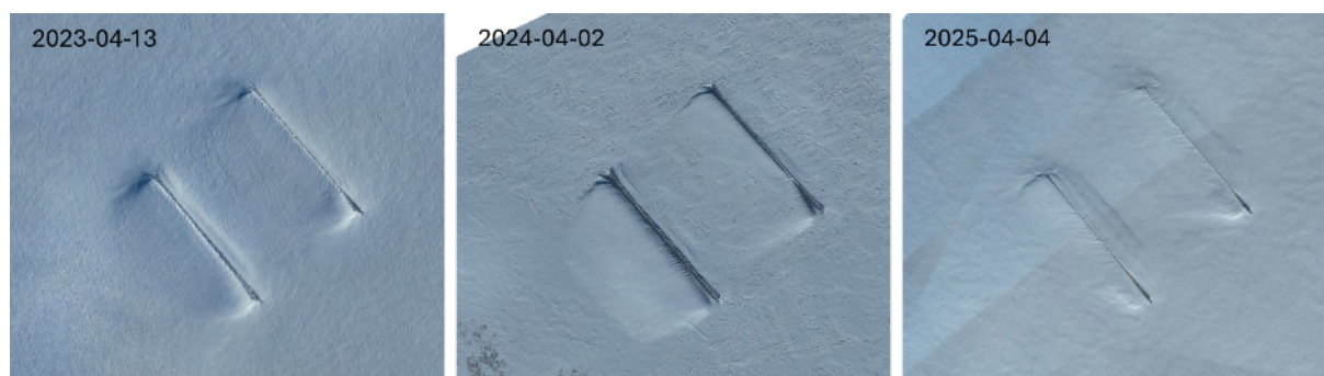
Figure 6 Late winter accumulation around the snow fences for each winter.
