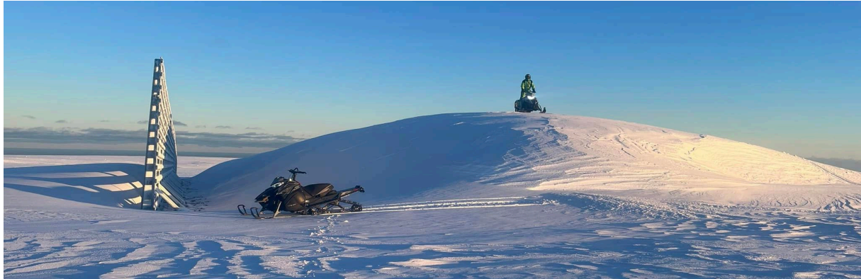
Figure 8 Testing of two rows of 5 m high and 150 m long snow fences started in winter 2022. Photo: Veðurstofa Íslands, January 15 th 2023.
