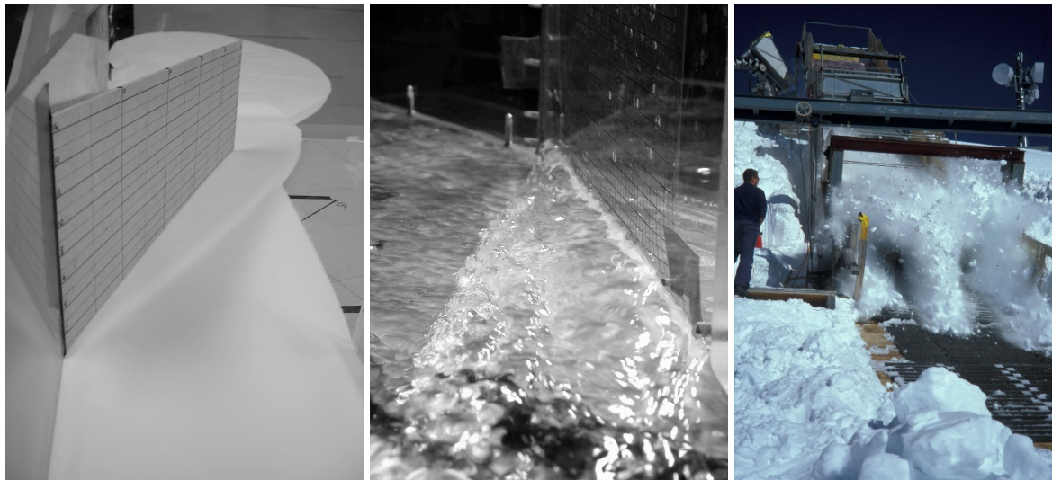
Figure 3 Left and middle: Small scale laboratory experiments showing photographs of oblique shocks in a granular flow at Froude number 5, looking downstream onto the deflector, and in water flow at Froude number 4.5, looking upstream into the flow along the deflector (Hákonardóttir and Hogg, 2003). Right: A photograph of snow experiments at Weissfluhjoch in Davos. An avalanche launched over two 0.6 m high mounds. The snow is deflected both over and around the mounds and an interaction between jets launched from adjacent mounds takes place (Hákonardóttir et al., 2003c).
