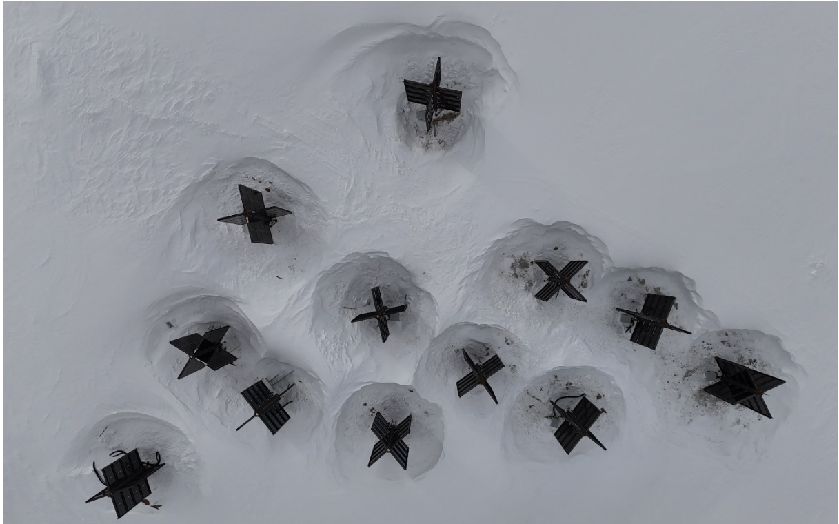
Figure 2 View of the vortex effect shown from above (test field Sölden, Austria) – similar to a protective mountain forest
