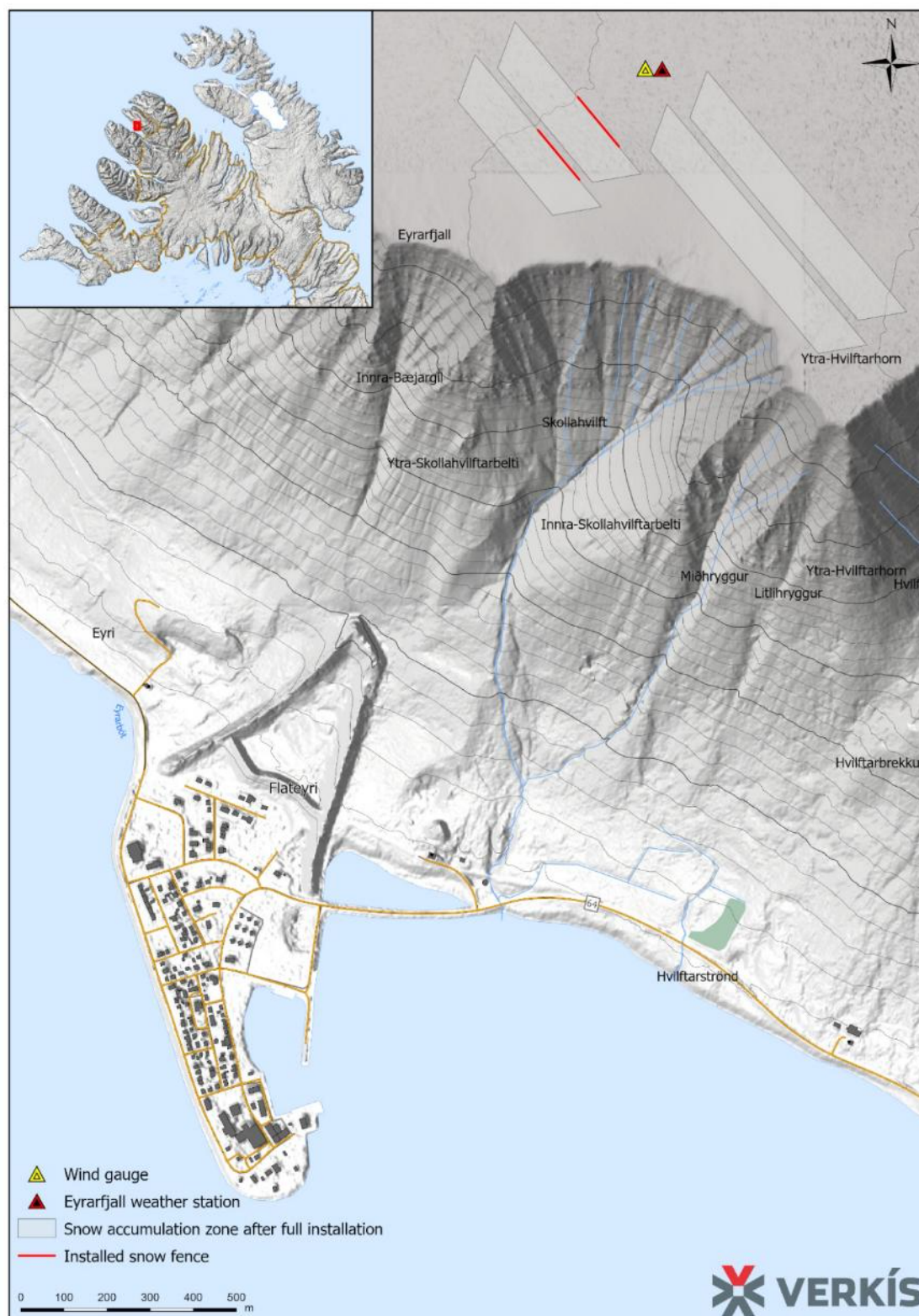
Figure 1 An aerial view of Eyrarfjall, above Flateyri. Shown on the Figure: The location of the installed snow fences, key instruments, proposed snow accumulation zones after full installation and the gullies above Flateyri village.
