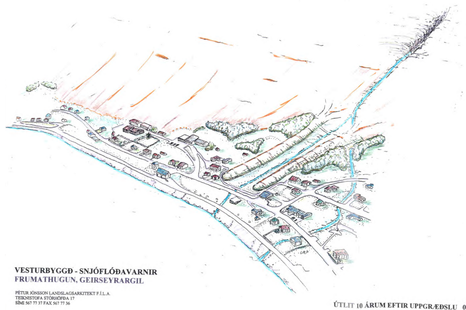
Figure 3. Sketch of previously proposed defence measures (reproduced from VST/NGI (1998)).
