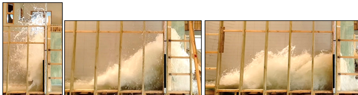
Figure 4 Stills from slushflow experiments at a dimensional scale of 1/10. Supercritical water flow at a Froude number of approximately 5 hits a 1 m high catching dam. The pictures show the different flow stages of the interaction. Left: The initial violent splash. Middle: The semi-steady fountaining, approximately 1.25 s after initial impact. Right: Hydraulic jump, approximately 2 s after initial impact (Hákonardóttir and Andrésdóttir, 2019; Hákonardóttir et al., 2024a).
